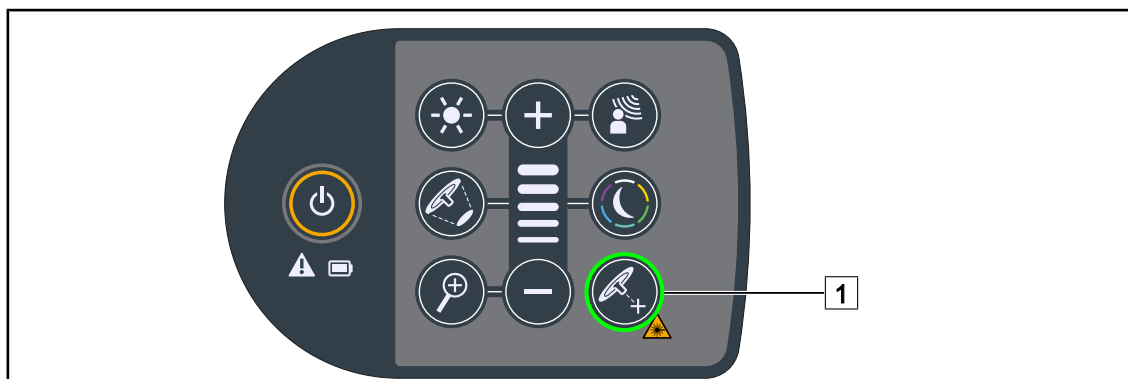
Fig. 65: Enabling the laser positioning assistance function via the keypad
