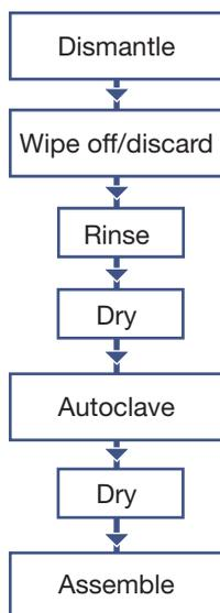
Autoclaving will reduce the lifetime of the expiratory cassette and is not recommended as a cleaning method.
