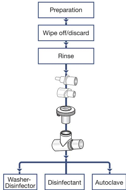
Only the Aerogen Pro Nebulizer unit, T-piece and neonate adapters can be autoclaved.
