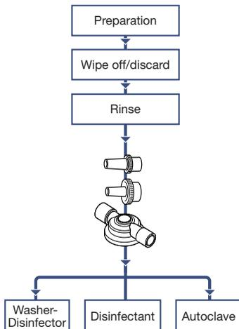
Only the T-piece and nipples can be autoclaved.
