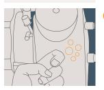
Tap module and tubing with hand to remove bubbles.
