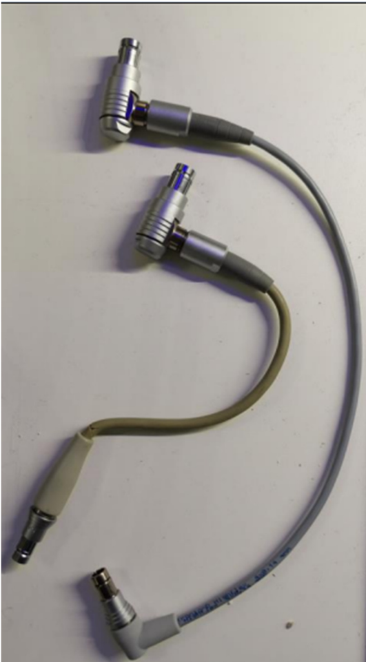
Figure 1 – Previous version of (short) cable (L), Current version of (long) cable (R). There are notable differences in length and in the end plug of the cables.
